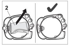
To suck wet dirt, first remove the paper filter bag (2).
